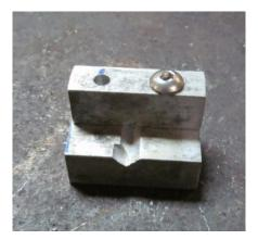
The last step is to make a cut with the band saw along the inner face of the upper block as shown to just beyond the edge of the "V". For at least this right-handed smith, I like the upper block on the left so that the piece to be cut off is on the right – where I can catch it as it is parted from the stock material.
